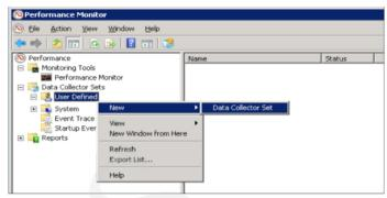
Fig. 1 Perfmon main window. A new data collector set is going to be defined
