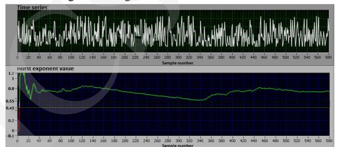
Fig. 5. The charts of the VoIP traffic with a small load and the Hurst exponent value obtained using the absolute value method.
