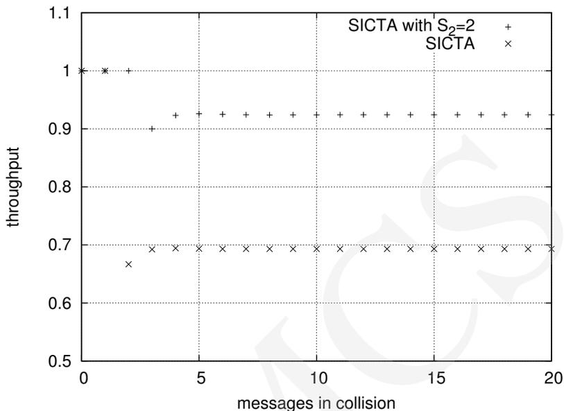
RYSUNEK 2. Performance of collision resolution with SICTA.
