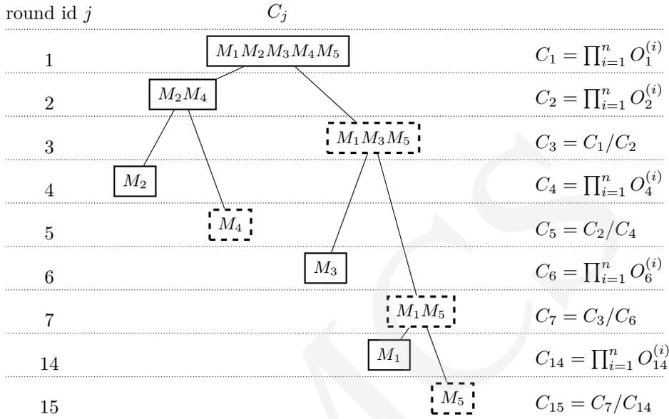
RYSUNEK 1. Exemplary binary collision resolution tree with successive inference cancellation (SICTA). In rounds 1,2,4,6 and 14, the ciphertexts  $O_j$  are transmitted, and  $C_j$  is computed using these ciphertexts. In rounds 3,5,7 and 15, no data is transmitted and  $C_j$  is computed using the data from the parent node and the sibling node.
