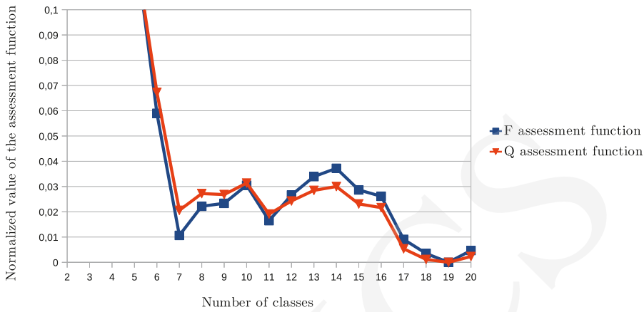
FIG. 4. Graph showing the dependence of the functions F and Q on the number of classes for the building_1 image. The function values were scaled to the interval of [0; 1] . The chart shows only the [0; 0, 1] range in order to make local minima more visible.
