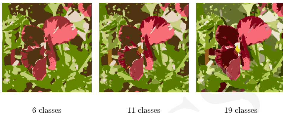
FIG. 3. Segmentations of flower_3 test image chosen based on the F and Q function values. The following parameters were used during the over-segmentation reduction – clustering method: Ward's minimum variance , watershed attributes: average and standard deviation , standardization: none .
