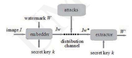
Fig. 1. Typical watermark system model.
