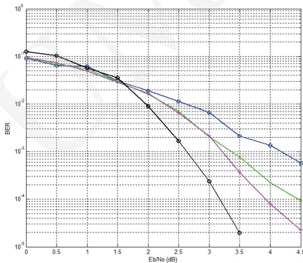
Fig. 6. Bit error rate for  $[75, 150]$  code (blue),  $[500, 1000]$  code (green),  $[1875, 3750]$  code (purple) and  $[250, 500]$  code (black), all based on the Radford M. Neal random constructions [16] with the code rate  $R_C = 1/2$ .
