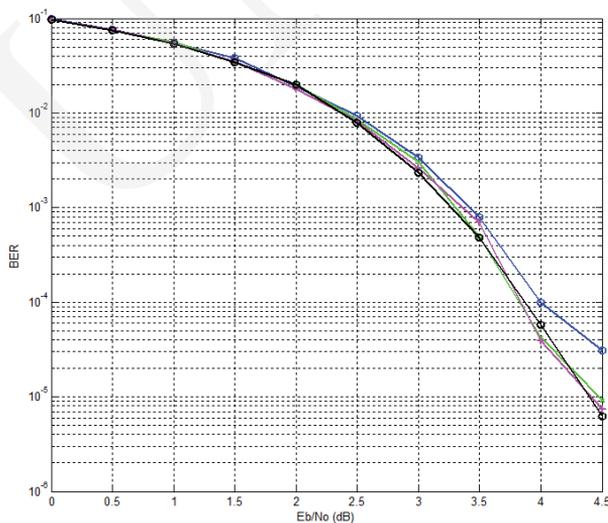
Fig. 4. Bit error rate for  $[250, 625]$  code (blue) based on  $A(6, 5)$ ,  $[1250, 3125]$  code (green) based on  $A(7, 5)$ ,  $[1250, 3125]$  code (purple) based on  $A(8, 5)$  and  $[1250, 3125]$  code (black) based on  $A(9, 5)$
