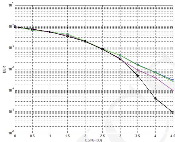
Fig. 3. Bit error rate for  $[50, 125]$  code (green) based on  $D(6, 5)$ ,  $[50, 125]$  code (blue) based on  $D(7, 5)$ ,  $[250, 625]$  code (purple) based on  $D(8, 5)$  and  $[1250, 3125]$  code (black) based on  $D(9, 5)$
