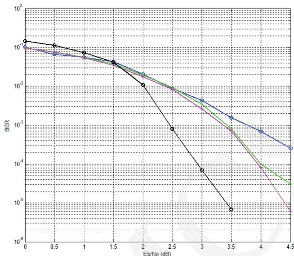
Fig. 7. Bit error rate for  $[50, 125]$  code (blue) based on  $\widetilde{D}(6, 5)$ ,  $[250, 625]$  code (green) based on  $A(6, 5)$ ,  $[1250, 3125]$  code (purple) based on  $A(9, 5)$  and  $[375, 625]$  code (black) based on  $\widetilde{D}(5, 5)$
