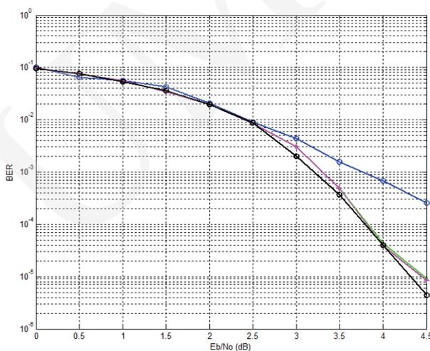
Fig. 2. Bit error rate for  $[50, 125]$  code (blue) based on  $\widetilde{D(6, 5)}$ ,  $[1250, 3125]$  code (red) based on  $\widetilde{D(7, 5)}$ ,  $[1250, 3125]$  code (purple) based on  $\widetilde{D(8, 5)}$  and  $[1250, 3125]$  code (black) based on  $\widetilde{D(10, 5)}$
