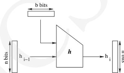
Fig. 2. Compression function of a hash function
