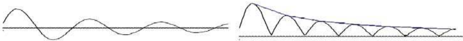
Fig. 1. Left: Cross-section of one CWT_{a,b} scale. Right: Cross-section of one |CWT_{a,b}| scale and its contour (smoothed version).
