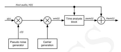
Fig. 1. Watermark embedder block diagram.
