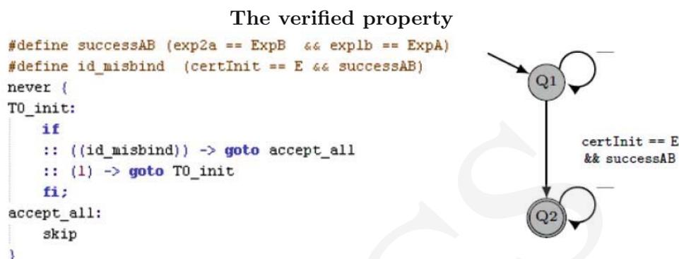
Fig. 5. Büchi automaton constructed from the *LTTL* logic formula  $\diamond id\_misb$  (identity misbinding attack is possible). Specification in the *Promela* code (left) and graph representation (right).
