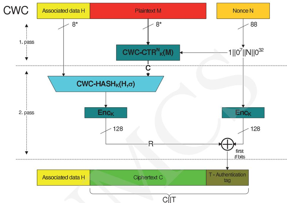
Fig. 5. CWC authenticated encryption scheme.
