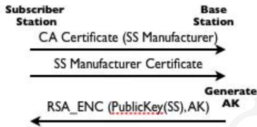
Fig. 4. Station Authentication Process.
