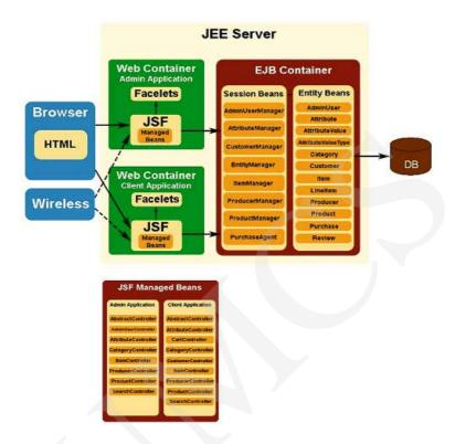
Fig. 1. System architecture.
