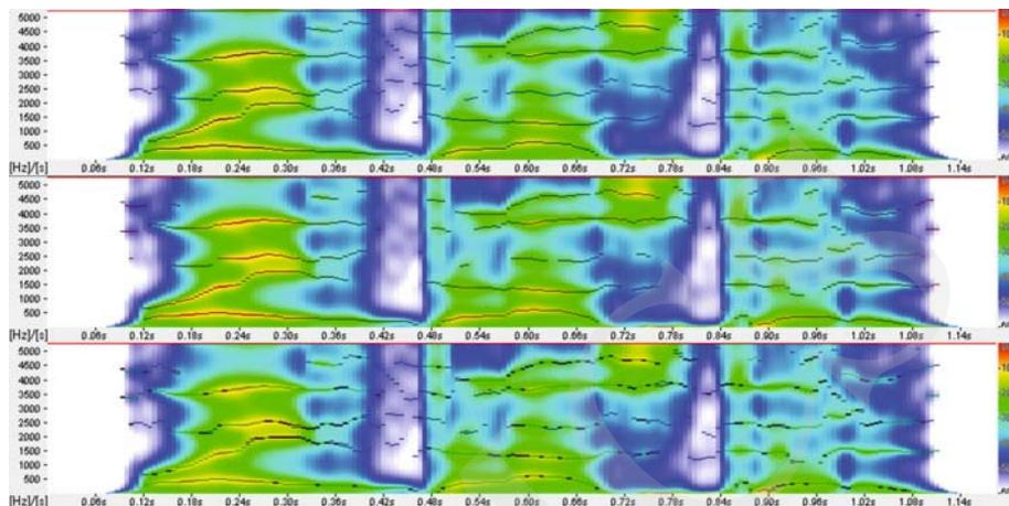
Fig. 6. Formant paths computed with LP  $p=24$  for the utterance 'wave blaster'. On the top - the root extracting formant paths, in the middle - the peach picking formant paths and at the bottom - both of them (overlapping).
