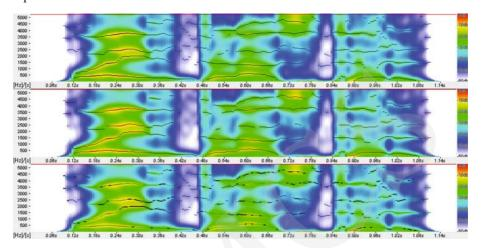
Fig. 6. Formant paths computed with LP p=24 for the utterance 'wave blaster'. On the top - the root extracting formant paths, in the middle - the peach picking formant paths and at the bottom - both of them (overlapping).
