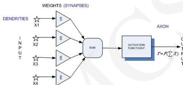
Fig. 1. A scheme of an artificial neuron.
