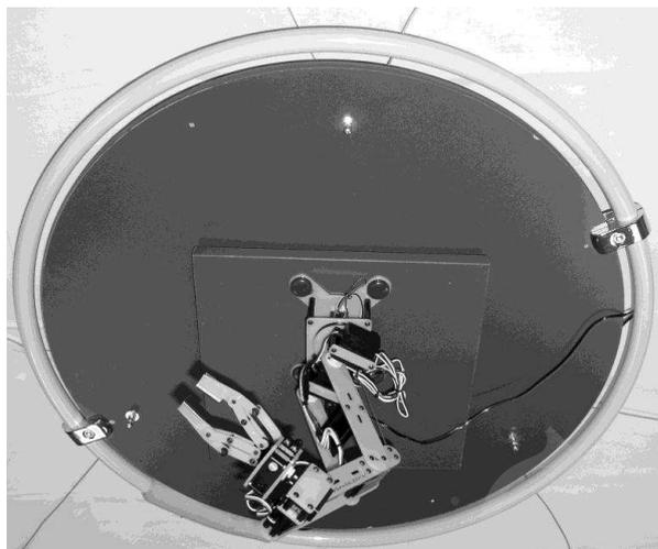
Fig. 6. Educational robotic arm as the end-effector of the cable manipulator
