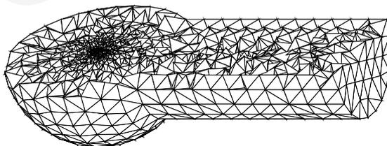
Fig. 8. A cylinder united with a part of the sphere with a symmetrical sharing plane -
