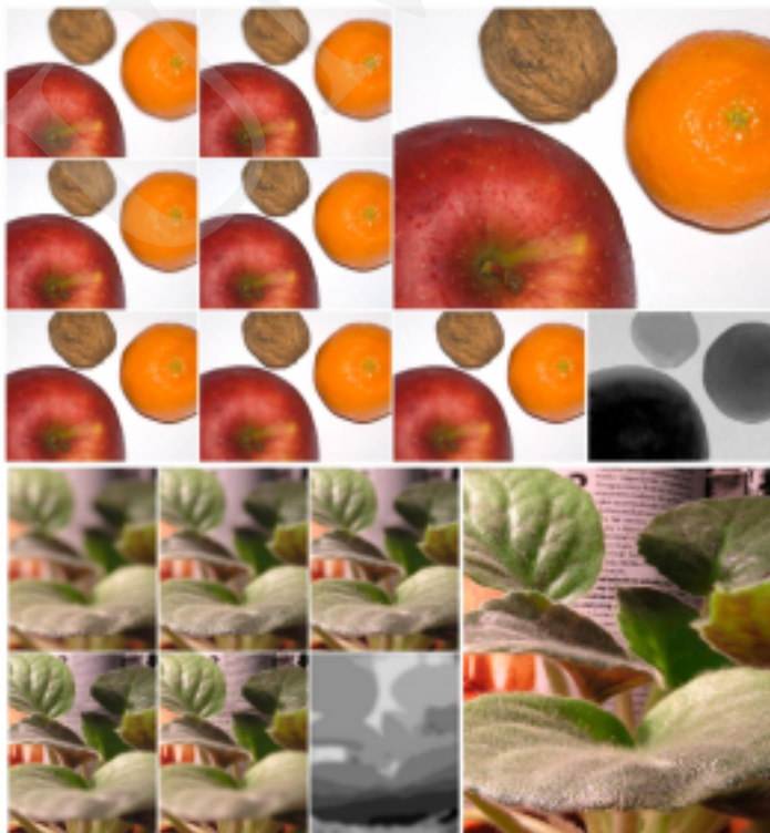
Fig. 3. Multifocus Image Fusion example sets. Small images are part of the original multifocus image set; last small, blurred image is the Height Map; large image is the fused image
