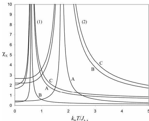
Fig. 4. Magnetic susceptibility  $\chi_X$  ( $X = A, B$ ;  $\chi_C = \chi_A + \chi_B$ ) vs. reduced temperature  $k_B T / J_{AA}$  for diluted ( $x = c_C$ ) binary amorphous structure  $(A_p B_{1-p})_x C_{1-x}$  with  $z_A = z_B = 3$ , and two sets of parameters described above in the text
