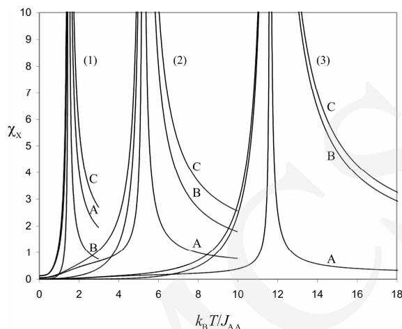
Fig.3. Magnetic susceptibility  $\chi_X$  ( $X = A, B$ ;  $\chi_C = \chi_A + \chi_B$ ) vs. reduced temperature  $k_B T / J_{AA}$  for non-diluted ( $x = 1$ ) amorphous structure  $(A_p B_{1-p})_x C_{1-x}$  with  $z_A = 2, z_B = 4$ , and three sets of parameters described above in the text
