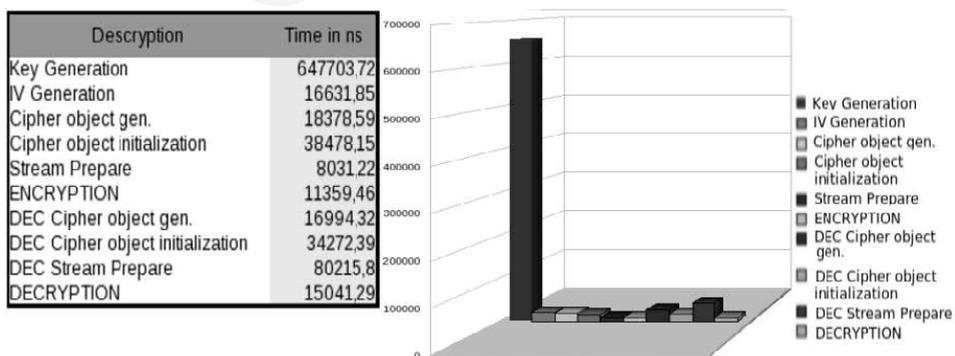
Fig. 6. Time consumption of the Triple DES algorithm
