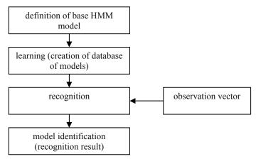
Fig. 1. The HMM based recognition process
