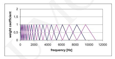
Fig. 2. The characteristics of the applied filter set (20 filters covering 0-10969 Hz range)
