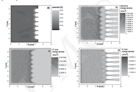
Fig. 7. The plasma potential and charge density distribution at the final stage of simulation (after 3150 time steps)
