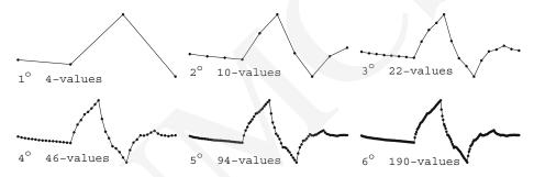
Fig. 8. Consecutive approximations of the Daubechies 2 wavelet obtained by the recursive algorithm
