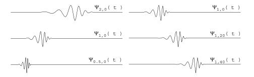
Fig. 2. Exemplary functions from the wavelet family  $\psi_{a,b}(t)$
