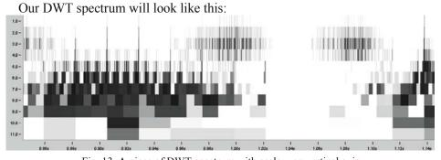
Fig. 13. A piece of DWT spectrum with scale a on vertical axis
