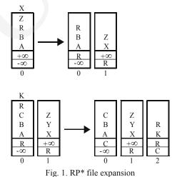
Just as this bucket load reaches some critical level, a split is performed and new bucket with number 1 is created. Generally, newly created bucket gets number (logical address) M, if the file consists of M buckets while split is initiated.
