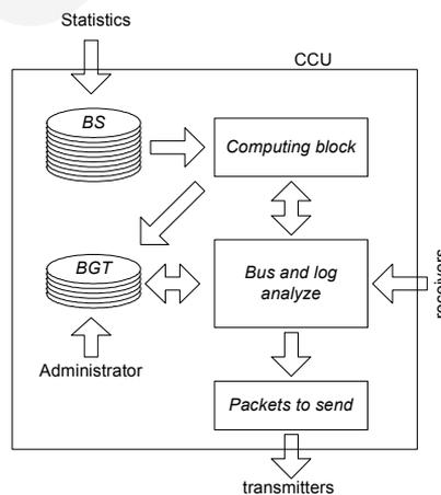
Fig. 6. CCU structure
