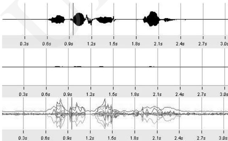
Fig. 1. From the top: input signal, prediction error  $e(n)$ , changes of 20  $\alpha$  coefficients for the sample „mleko jest zdrowe”. Window width – 29 ms. The screenshot comes from a program created by the authors of this paper
