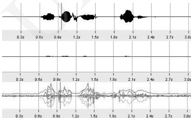
Fig. 1. From the top: input signal, prediction error  $e(n)$ , changes of 20  $\alpha$  coefficients for the sample „mleko jest zdrowe”. Window width – 29 ms. The screenshot comes from a program created by the authors of this paper
