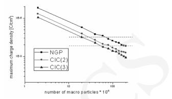
Fig. 6. Maximum deviations from the zero of charge density averaged over five middle grid layers versus the number of macro particles for three methods of charge distribution
