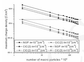
Fig. 9. Comparison of maximum deviations of charge density averaged over five middle grid layers for the two plasma concentration values (10<sup>10</sup>[cm<sup>-3</sup>] and 10<sup>11</sup>[cm<sup>-3</sup>])
