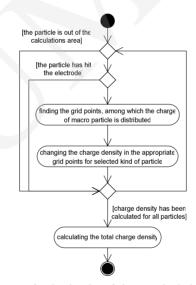
Fig. 1. The diagram for the density of charge calculation procedure [3]
