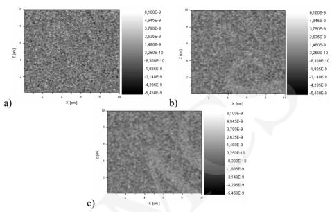
Fig. 4. The cross-sections of charge density distributions (in C/cm³) calculated by different methods for 20 mln of macro particles: a) NGP, b) CIC (2), c) CIC (3)
