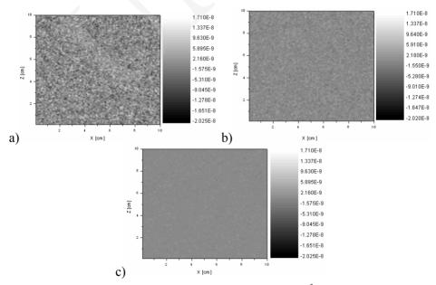
Fig. 5. The cross-sections of charge density distributions (in C/cm³) calculated by the NGP method for different number of macro particles: a) 2 mln, b) 20 mln, c) 200 mln
