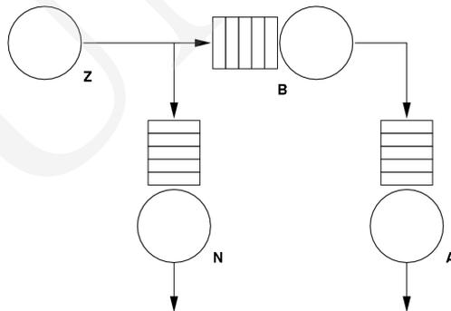
Fig. 2. A queuing model of the RED mechanism
