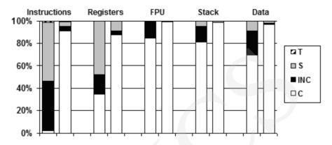
Fig. 3. Fault susceptibility of two versions of FFT algorithm
