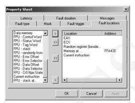
Fig. 1. FITS window for defining fault injections
