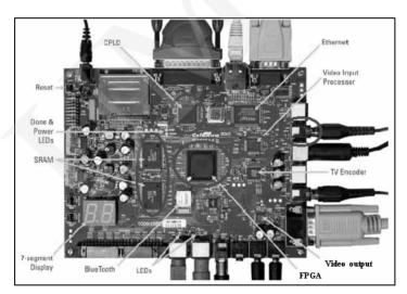
Fig. 3. Components of the FPGA development board used in the second-level node
