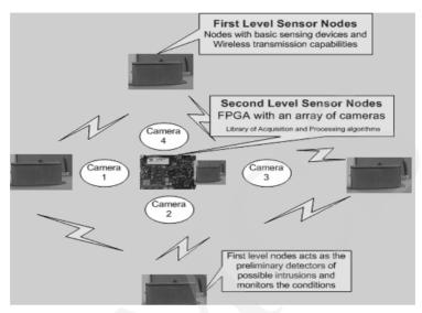
Fig. 1. Basic structure of the developed sensor network
