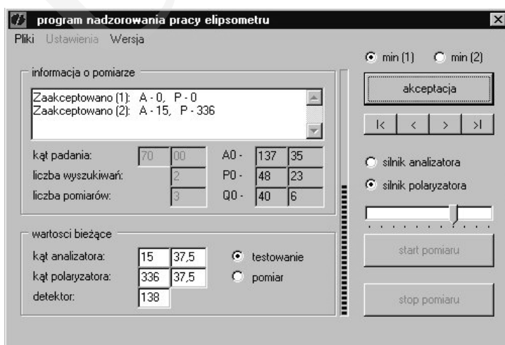
Fig. 4. Ellipsometer operation management program – graphical interface
