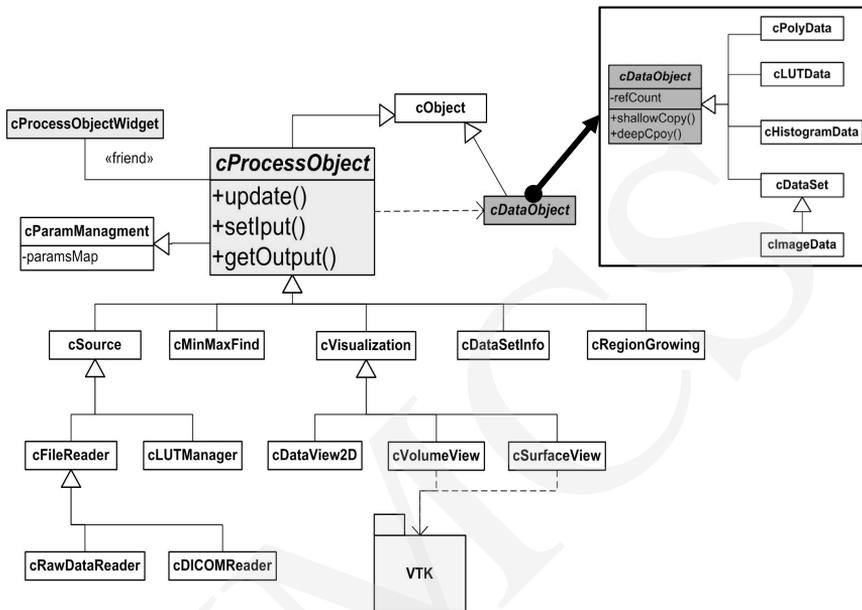
Fig. 3. *SemiVis* framework package and class diagram
