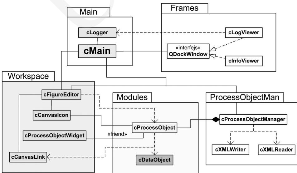
Fig. 2. General *SemiVis* framework package and class diagram
