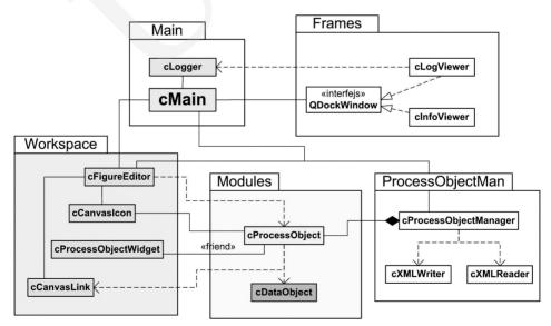
Fig. 2. General SemiVis framework package and class diagram
