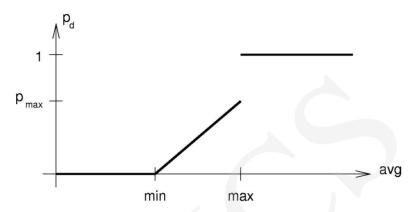
Fig. 2. The drop probability  $p_d(avg)$  in the RED mechanism
