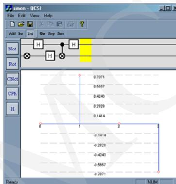
Fig. 5. Simulation of Deutsch algorithm in QCSI
