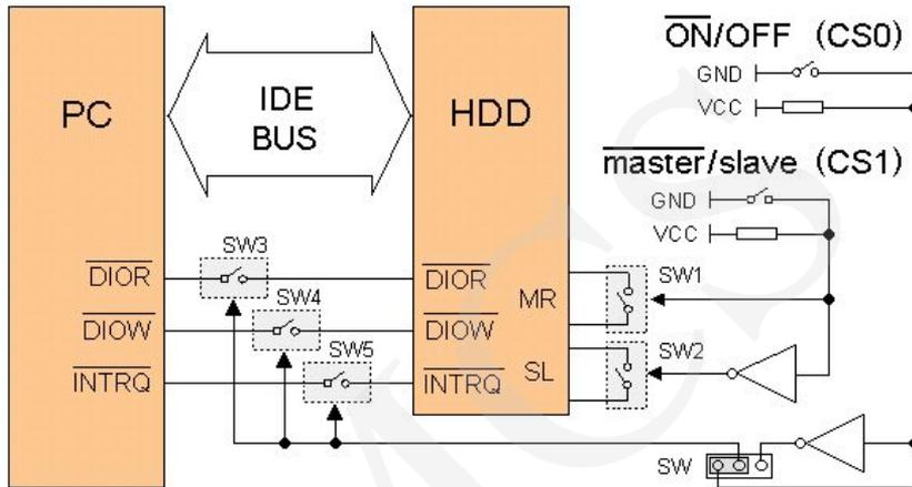
Fig. 3. Circuit scheme of the HDD switch
