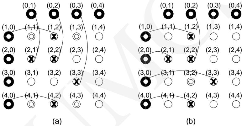
Fig. 3. Local (a) and global (b) reconfigurations
