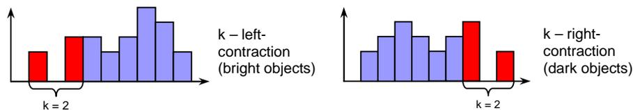
Fig. 3. Examples of 2-left-contraction (a), 2-right-contraction (b)
