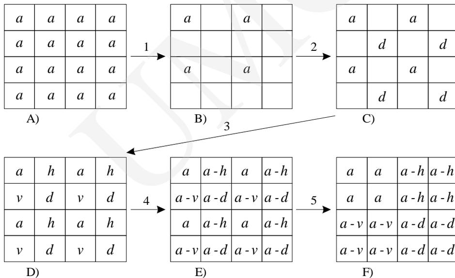
Fig. 1. The scheme of dyadic median decomposition
