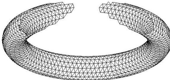
Fig. 7. Unstructured mesh on a torus – mesh construction
