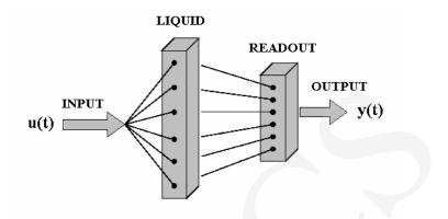
Fig. 1. Scheme of the Maass' LSM
