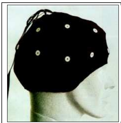
Fig. 2. Mindset MS-1000 EEG system Electro-Cap
